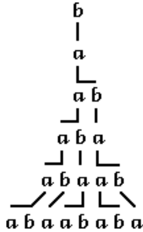
Figure 1.3: Example of a derivation in a DOL-system
